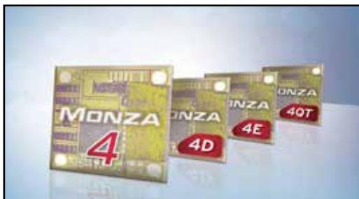
Among Impinj products is the Monza 4 family of RFID tag chips, which deliver privacy, performance, and memory benefits that address even the most challenging of RFID applications. The chips provide the best sensitivity combined with excellent interference rejection, support for omni-directional antennas (True3D antenna technology), innovative privacy features (QT technology), and expanded memory options.
